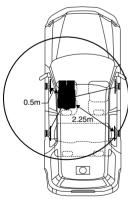
The sound is uneven because the distance between the listening position and the different speakers is different. The difference in the distance between the front left and rear right speakers is 1.75 meters (68-3/4").
